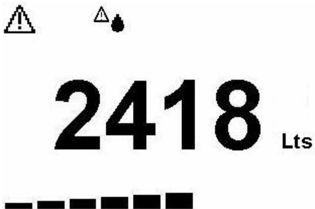
Figure 7 LCD – Leak Error Alarm
