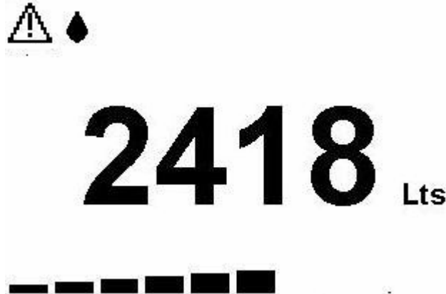
Figure 6 LCD – Leak Alarm
